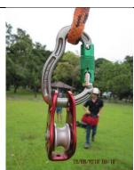
Step 2. Tie the throw line to spliced eye end on approved arborists climbing rope and pull through over palm to receive eye end
